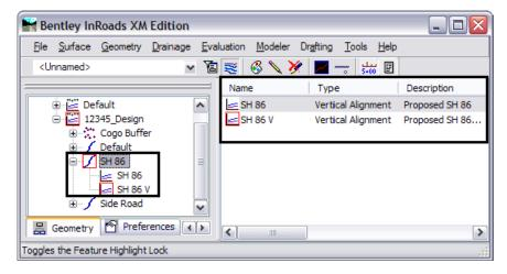
**Note:** Only one horizontal alignment can be active at a time. Being *active* specifies the alignment to be modified, displayed, or defined by default in dialog boxes.
