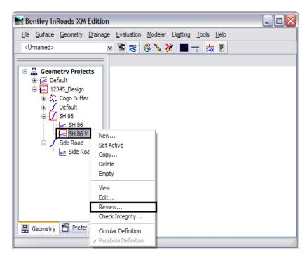
4. Review the *Vertical* alignment SH 86 V associated with horizontal alignment SH 86.
