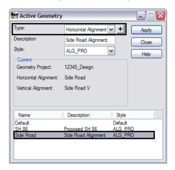
9. Select **Geometry > Active Geometry**. The *Active Geometry* dialog will appear.
