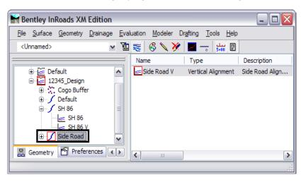
13. Select **Geometry > Review Horizontal** for a textual display of the active alignment. When reviewing an alignment, a temporary dynamic display is shown in MicroStation representing the location of the alignment being reviewed.
