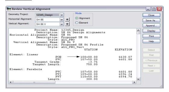
If the horizontal and vertical stationing are not sychronized it will cause confusion in the design and construction processes. Is the stationing for the horizontal and vertical alignments synchronized?
