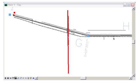
19. In the Workspace Bar <**R**> (right-click) on the active alignment name. Note the *Active*, *View*, *Fit*, and *Review* commands are available from the short-cut fly-out menu.
